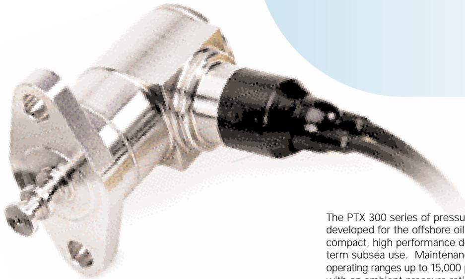
The PTX 300 series of pressure transmitters has been developed for the offshore oil and gas industries as a compact, high performance device for reliable and long term subsea use. Maintenance free, it is available with operating ranges up to 15,000 psi and is fully submersible with an ambient pressure rating up to 4000 psi.
