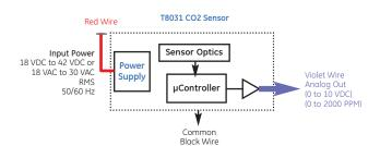
The T8041 is a  $\rm CO_2$  transmitter designed to be installed in HVAC return air ducts. This product offers simplicity in design and installation. Available with analog 0-10V output only. Includes mounting hardware and installation instructions
