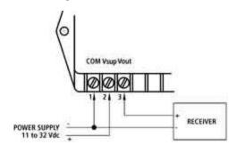
Terminal 1 is common to both the DC power supply and the output signal.
