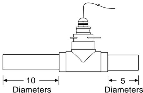
In the larger sizes, the length provided is less than ten diameters upstream and five downstream. It is not advisable to connect directly to the end of these fittings with a flow-disturbing device such as a valve or elbow. If possible, straight pipe should be added to these fittings.
