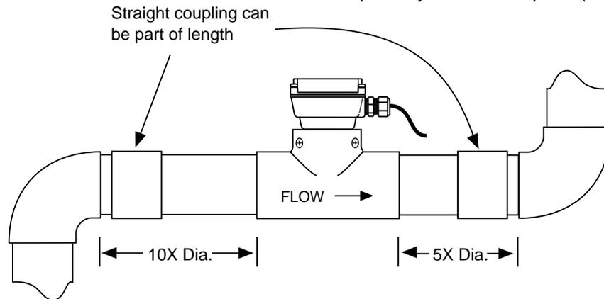
**Piping Conditions.** In general, the standard practice of installing the meter with five diameters of straight pipe upstream and three downstream is recommended. However, it is possible under some circumstances to operate with less, particularly if the meter is equipped with an optional internal flow straightener.
