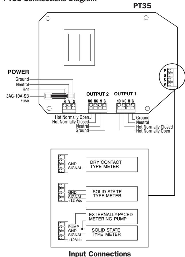
**Connect the Load.** Two output cords are provided for connection of 115 Vac loads. The unit can be hard-wired if necessary, using the terminals inside.
